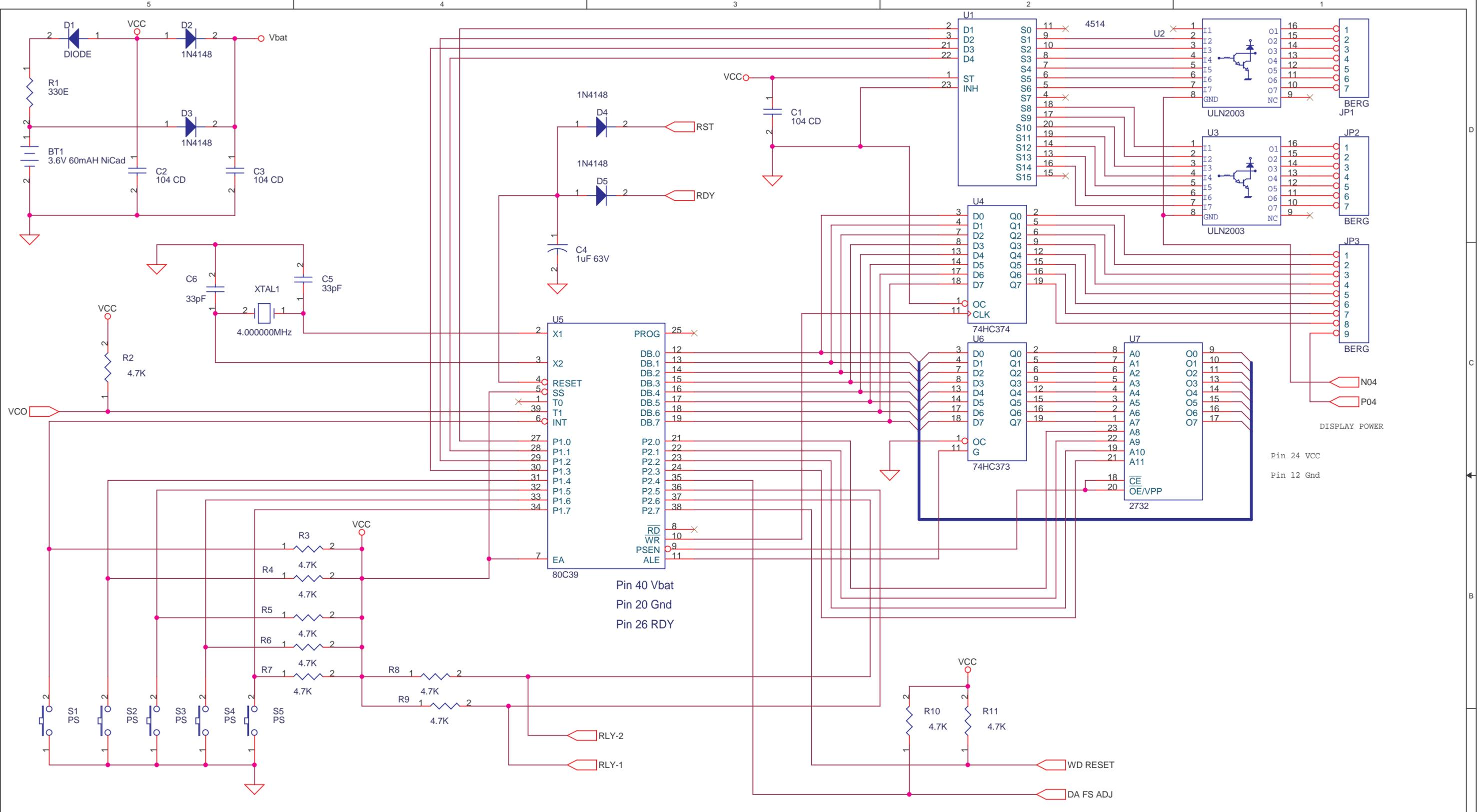
use 74HCT40XX chips in place of CD40XX for only 5V and high speed designs. Use Shrink sleeves and proper gauge of wire.
